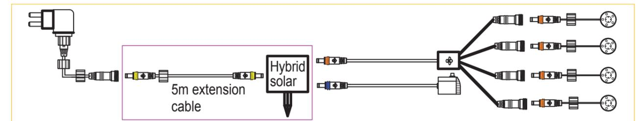
Connect the pump, LED lights and power adapter with hybrid solar panel. (see diagram)
