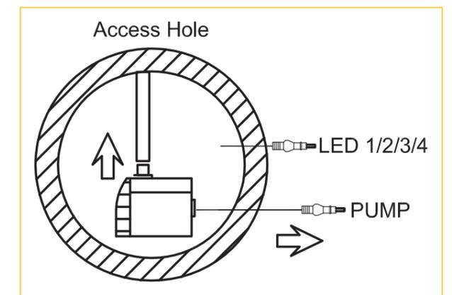
3.2 Connect pump and led light wth the power adapter (See diagram)
